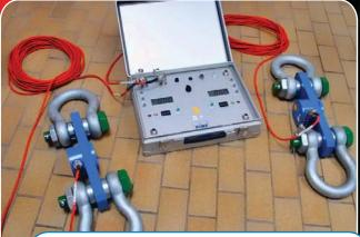
Shackles with load cells connected to digital load indicators mounted in an aluminium box
