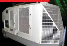
The Air Starter Unit series is a line of truck or trailer mounted continuous flow jet engine starting units
