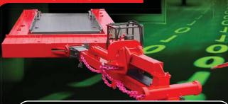
Aircraft Recovery Dollies for 'flat tires or damaged wheel' scenarios ensure rapid removal of an aircraft from runways.
