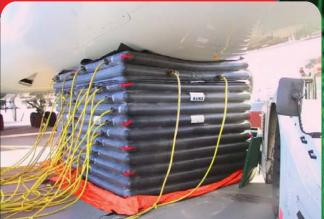
Pneumatic elevators to lift aircraft of any size in 'gear collapsed' scenarios. its made of thread fabric and rubber compound.
