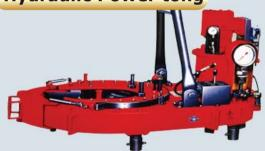
The drill pipe tong is applicable in the petroleum and mine drilling, it is safety and labor saving, and improving the working efficiency. Its using pneumatic power to shift and drive backup tong It is a integral mechanism during operation
