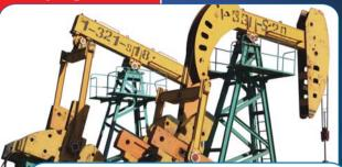
Pumping Units are among the commonly used ground-based machinery for petroleum extraction on oil fields.
