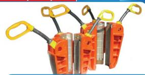
Full distribution of load through out the length of the slips which helps in preventing bottle necking damage of drill pipes.
