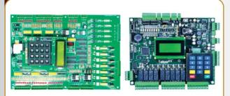
Latest MRAM memory technology to save events, failures and other data, Lead-acid battery charger.
