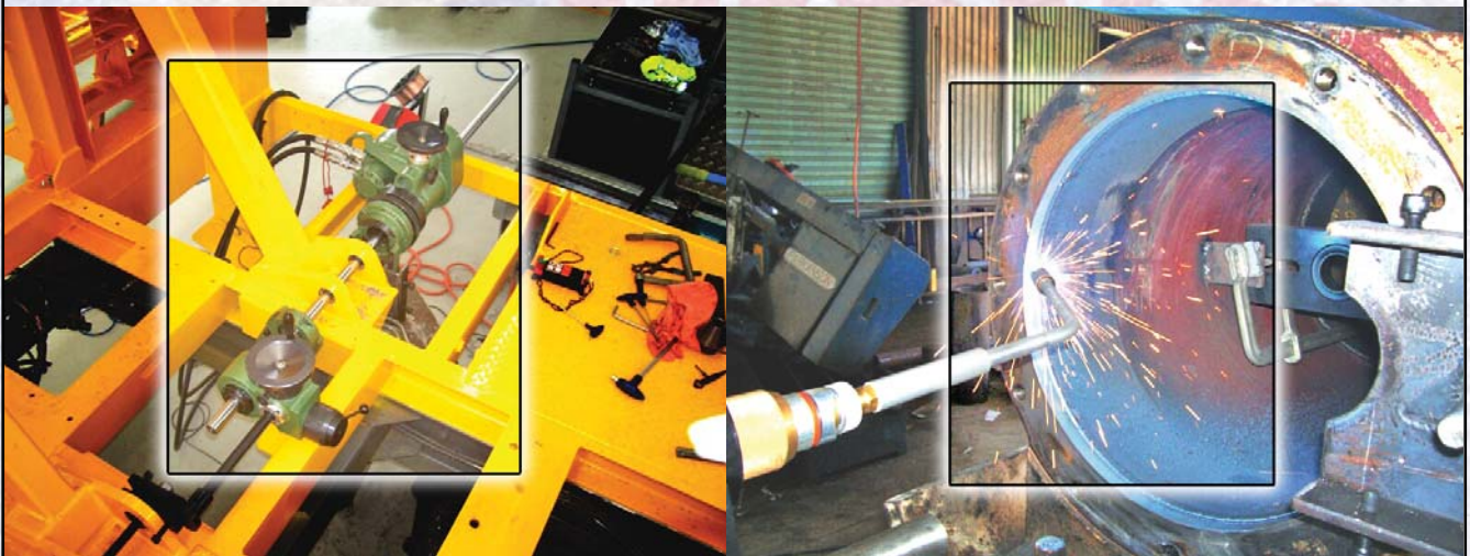
This mounting Flange was machined true as it had been distorted when the machine was fabricated.
