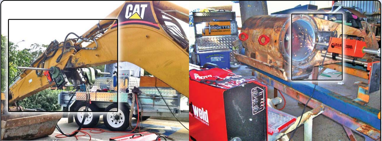
Backhoe Loader was in for a service when it was found some pivot bores were worn and the Clevis areas were bent.
