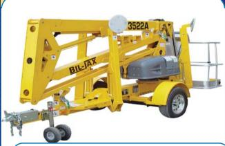
Trailer-mounted booms feature an outstanding operating envelope, making them ideal to reach jobs high and low. With easy-to-tow mobility and simple pictograph controls.
