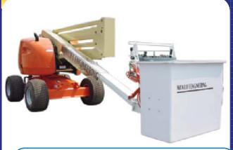
Electrically Insulated lifts are used where electrocution hazards exist such as working on any type of electrical wiring.
