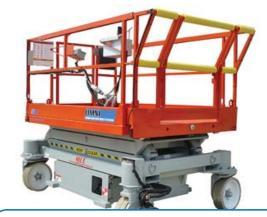
Unique Omni-Motion Drive System provides machine movement in all directions and machine rotation around its center point for optimum positioning.
