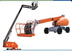
For use indoors or outdoors, Rolls through a commerical doorway, Removable cage converts unit to a 350 lbs material lift, With optional spanner kit.
